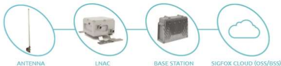
Figure 12: Main components of a Sigfox Base Station
